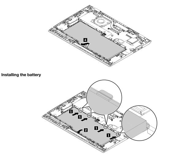
**Note:** Ensure that the battery tabs are inserted underneath the system board.
