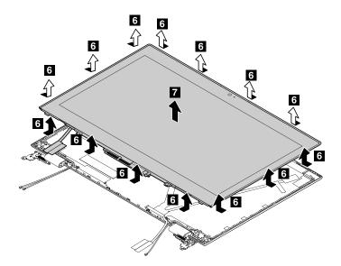
**When installing**: Ensure that the LCD panel assembly is hooked into place as shown in the following illustrations.
