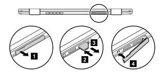
After you finish the servicing, ensure that you install the removed microSD card or nano-SIM card back into the computer.
